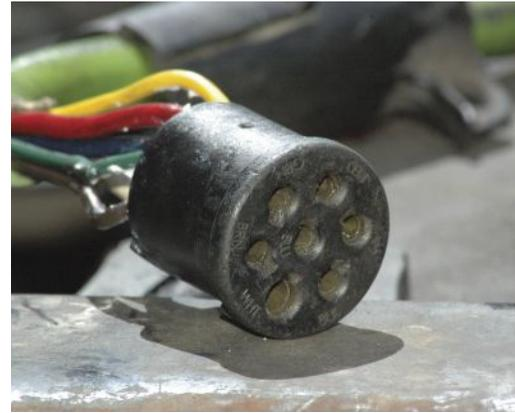
**All the energy needed for the trailer electrical system comes from the tractor. A logical place to look for bad connections or low-voltage problems is the seven-way pigtail cable.**
