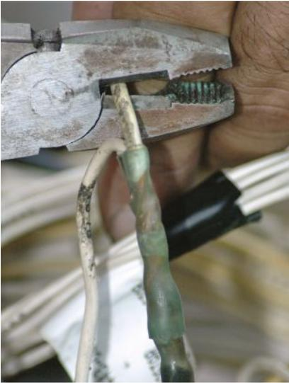
There are right and wrong ways of repairing and splicing wire. TMC's RP 186-Wire and Cable Repair Guidelines can help eliminate messes like this one.
