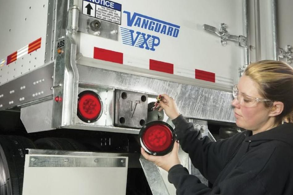
▼ Water, dirt, salt, and other road contaminants can enter a lamp or connector, providing an electrical path that can accelerate corrosion.
