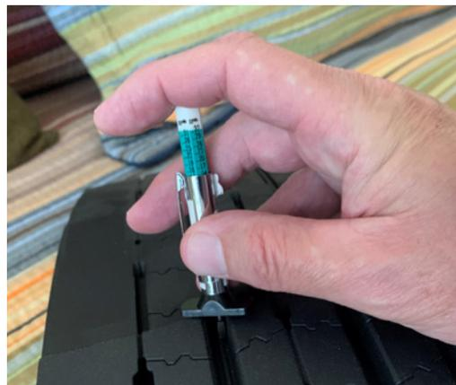
» Michelin Tire Care offers various program solutions to help fleets identify and address tire issues before they lead to safety risks. Tire inspections include the six critical factors that lead to poor tire performance, including mismatched tread depths. The 2020 North American standard out-of-service criteria from the CVSA says tires on the front steering axle must have 4/32" tread when measured in any two adjacent major tread grooves at any location on the tire.
