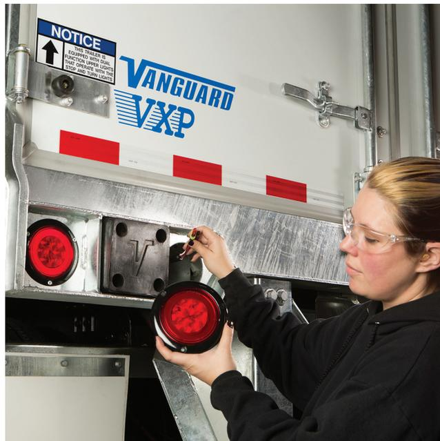
**Consider replacing conventional lamps with longer-life LED lamps that can offer better performance in environments where lighting systems are susceptible to corrosion.**
