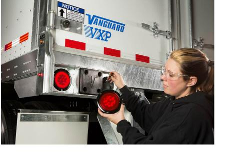
"Using good weather-resistant connectors such as AMP-compatible or other hard-shell connectors can help keep out corrosion at the connection point. Industry-standard type plugs, such as PL3 or P10, should be inspected regularly and dielectric grease should be used to protect the connection point," he says.
