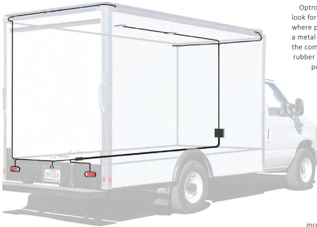
**Box truck wiring is generally simple and requires power to be supplied to stop, tail, turn, marker, and back-up lamps, and maybe interior dome lamps. But the addition of liftgates and pallet jack charging can make the system more complicated.**
