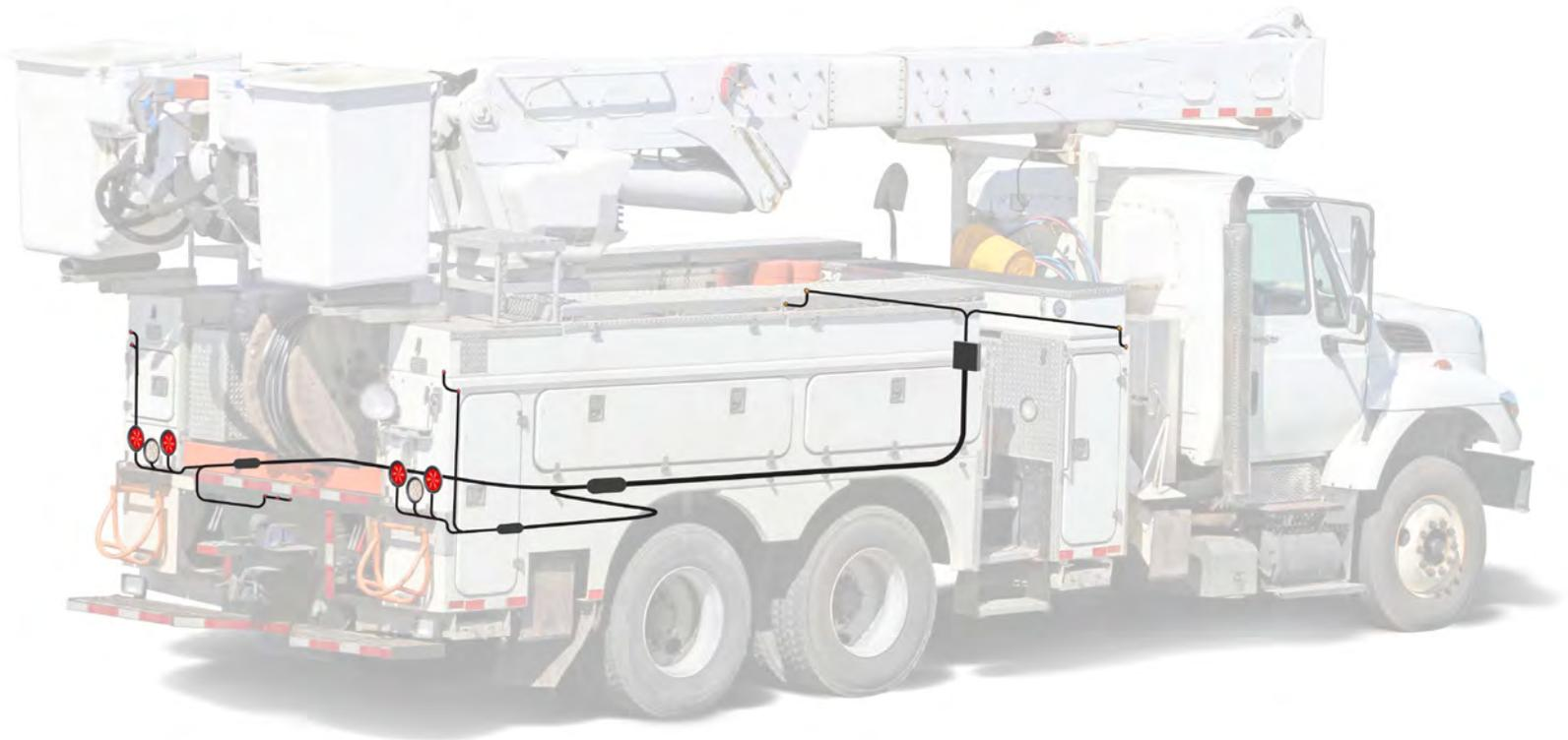
» Organizing wiring throughout a vehicle to indicate specific voltages per wire may alleviate issues when implementing new componentry.
